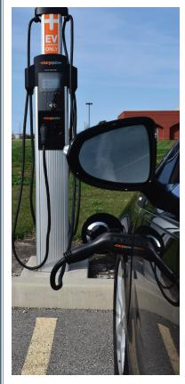
This electric vehicle charging station is a Level 2 commercial charging station capable of charging 2 vehicles at once. The cost to charge is \$0.20 / kWh and it might take 3-5 hours to add 40 miles of range to a vehicle. The MJM ChargPoint Station is the only listed public use EV charging station within 30 miles.
