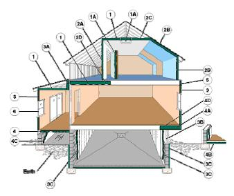
In unfinished attic spaces, insulate between and over the floor joists to seal off living spaces below.\*
